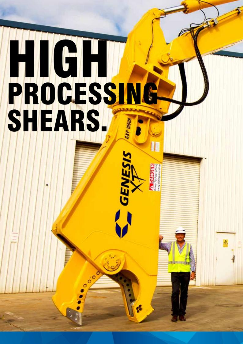
Newest additions to the fleet are the PC1250 and PC 850. One weighing 150 tonnes, the other 110 tonnes. The mechanical shears that are fitted to these machines are capable of cutting through 70mm steel plate and 1.5 metre steel beams, and can reach to heights of 24 metres.
